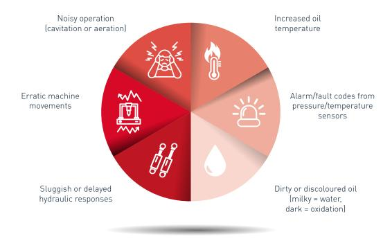
Contaminated hydraulic oil in an injection moulding machine is a serious issue that can lead to mechanical failures, reduced efficiency, and costly downtime. We understand the high cleanliness standards required for lubricants in plastic injection moulding. That's why our filtration oil fills are designed to meet those demands from the outset—giving you peace of mind that your machine is ready to perform from day one.
